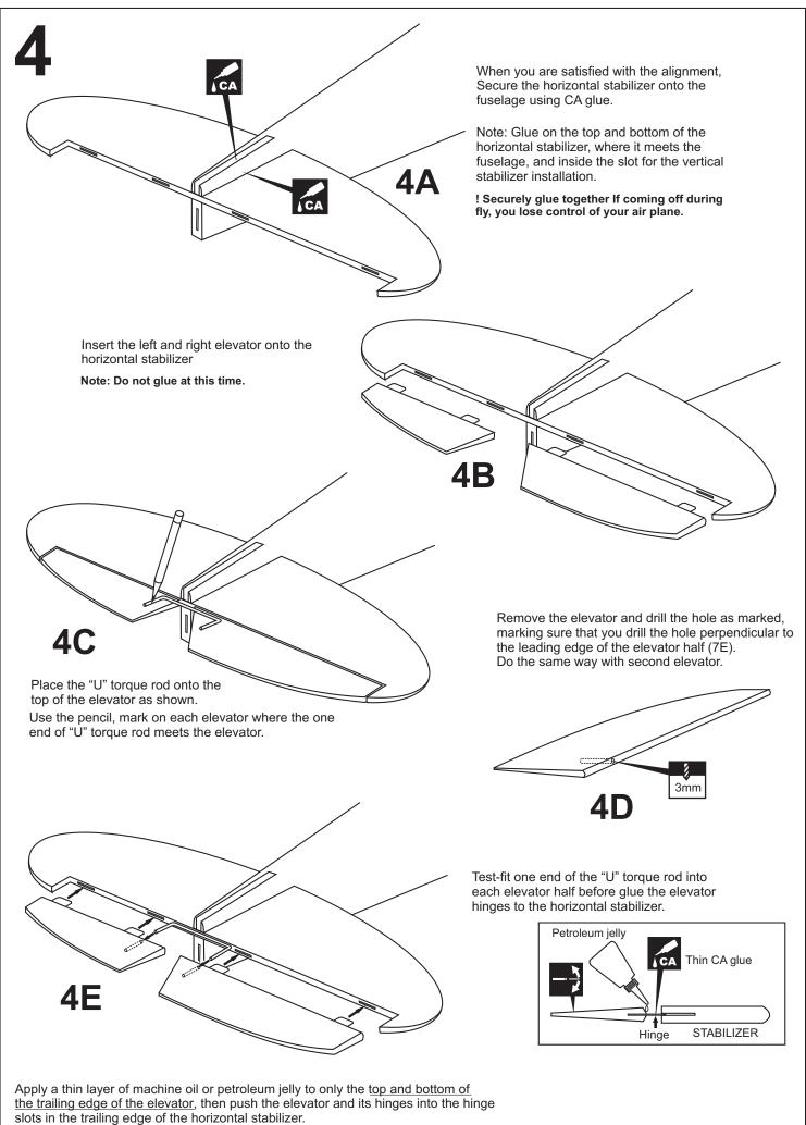
When satisfied with the and alignment, hinge the elevator to the horizontal stabilizer using CA glue.
